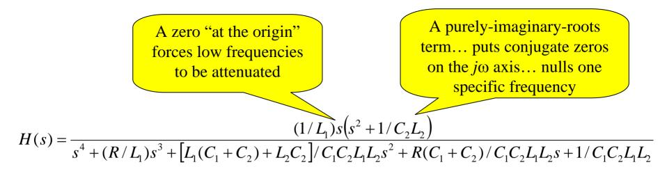
To see what this circuit can do we look at its frequency response. This is valid because all poles are in the region of convergence. (True for any <u>passive</u> RLC circuit)
