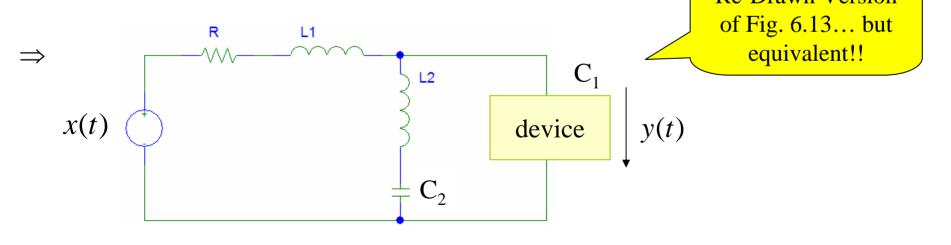
Now, replace "device" by its capacitor model and find the transfer function between:
