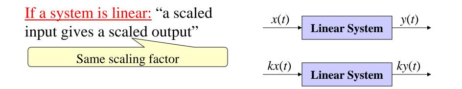
When superposition holds, it makes our life easier! We then can <u>decompose complicated signals</u> into a <u>sum</u> of <u>simpler signals</u>... and then find out how each of these simple signals goes through the system!!
