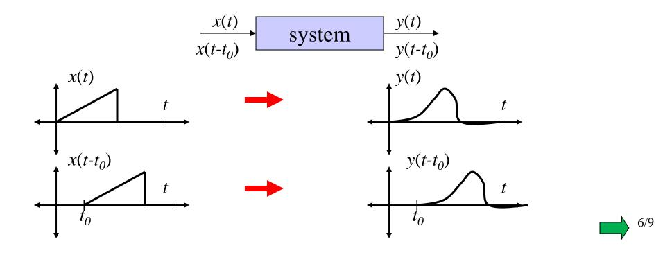
Systems described by Linear, Constant-Coefficient <u>Differential</u> Equations are <u>Continuous</u>-Time, Linear Time-Invariant (LTI) Systems
