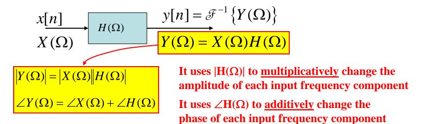
So...in general we see that the system frequency response re-shapes the input DTFT's magnitude and phase.
