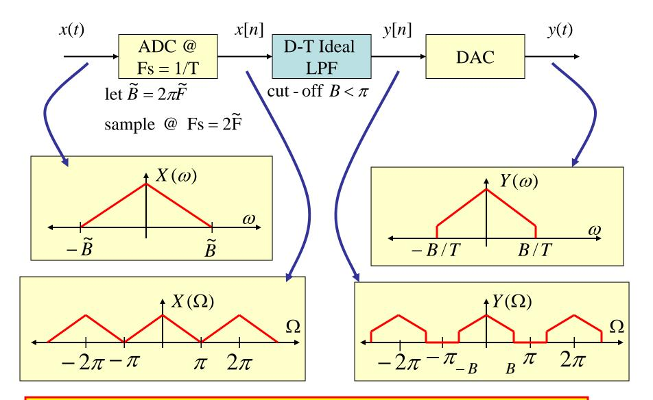
Whole System (ADC – DT filter – DAC) acts like an equiv. C-T system
