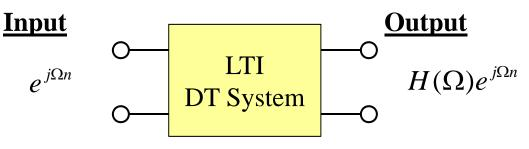
Input x[n] is a linear combo of sinusoids... the output is a linear combo:
