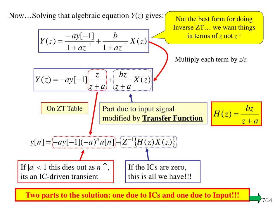
Ex.: Solving a Difference Equation using ZT: 1<sup>st</sup>-Order System w/ Step Input
