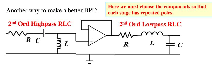
Although these ideas lead to workable circuits they are not necessarily the best... For one thing... they need inductors (which are big and can't be made in an IC!) There are other forms... See this link for the form used below.
