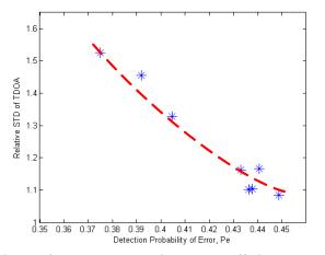
Figure 2: Results showing trade-off in the oneparameter & binary detection case.  $(SNR_1 = 10 \text{ dB}, SNR_2=40 \text{ dB})$
