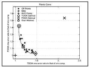
Figure 1: Trade-off between TDOA and FDOA accuracies as  $\alpha$  is varied for compression ratio 3:1 and  $SNR_1 = 15$  dB &  $SNR_2 = 15$  dB; symbol  $\Box$  denotes the operational point ( $\alpha$ =0.5) closest to that without compression.
