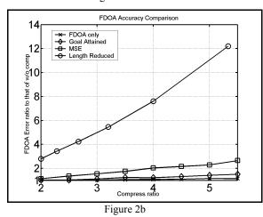
Figure 2: Effect of compression ratio on (a) TDOA and (b) FDOA performance. A comparison is also made to the case of simply sending less data ("Length Reduced") rather than compressing the data.
