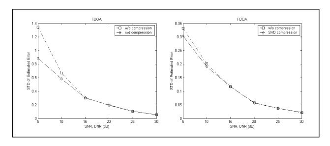
Figure 4: Simulation results showing standard deviation of TDOA/FDOA estimation error for a simulated radar signal when compressed 89:1 using SVD-based compression of the full pulse matrix (i.e., without pulse elimination); in each plot the SNRs of the two cross-correlated signals are set equal to each other as they are varied over a range. For comparison, results are shown for the case of no compression.
