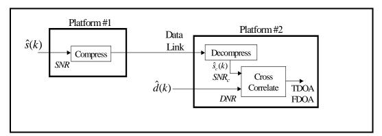
**Figure 1: System Configuration for Compression**
