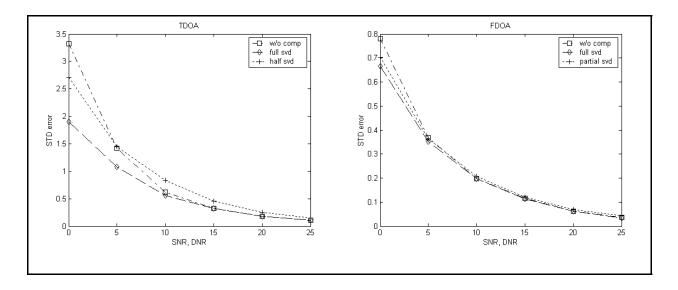
Figure 6: Simulation results showing standard deviation of TDOA/FDOA estimation error for a simulated radar signal when compressed using SVD-based compression. The three curves compare the cases (i) without compression, (ii) full SVD-based compression (i.e., no pulse elimination) with compression ratio of 89:1, and (iii) SVD-based compression where half of the pulses are eliminated to give a compression ratio of 105:1.
