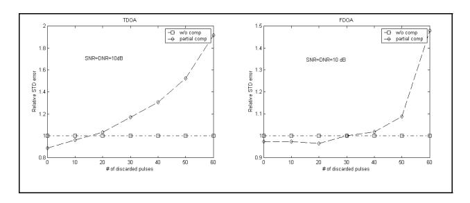
Figure 5: Simulation results showing the effect that discarding pulses has on the TDOA/FDOA estimation error standard deviation. The term "partial comp" means that SVD compression was done on a partial pulse matrix, after pulse elimination. For comparision, results are shown for the case without compression.
