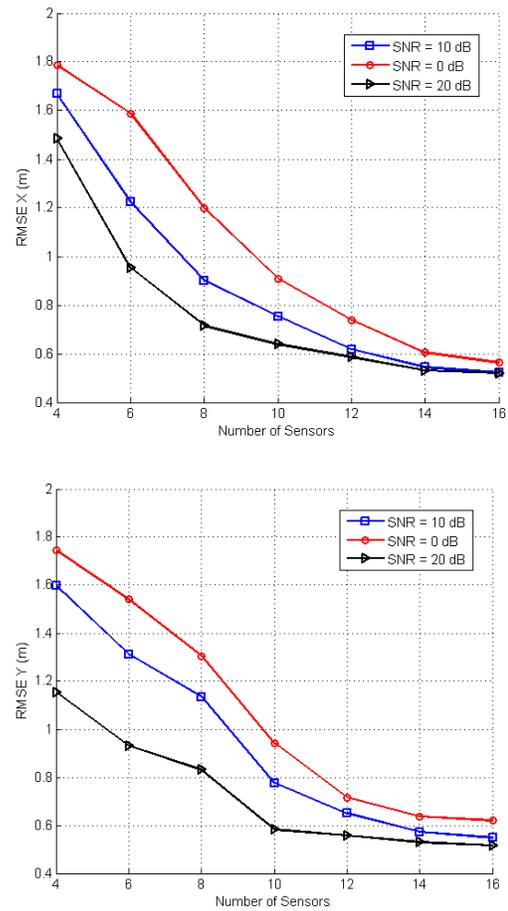
Fig. 1. RMS Error for X and Y location (in meters) versus Number of Access Points.
