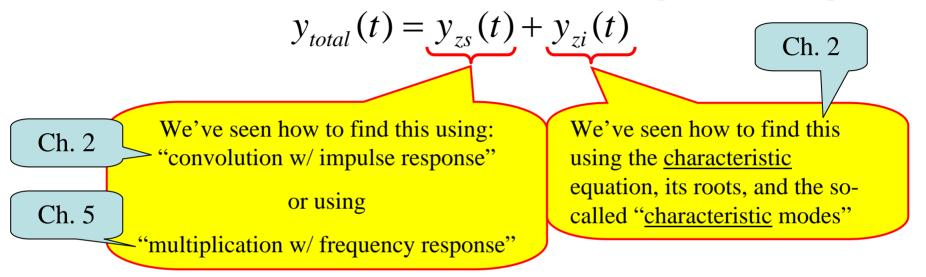
Here we'll see how to get  $y_{total}(t)$  using LT... ... get both parts with one tool!!! **First-order case:** Let's see this for a <u>1<sup>st</sup>-order Diff. Eq.</u> with a <u>causal input</u> and a <u>non-zero initial condition</u> just before the causal input is applied.
