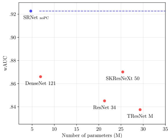
Figure 2. Performance in terms of wAUC versus model size (number of parameters) across different ImageNet pre-trained models building on the ResNet stem and SRNet noPC.
