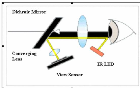
Figure 7. *Canon eye controlled focus.*
