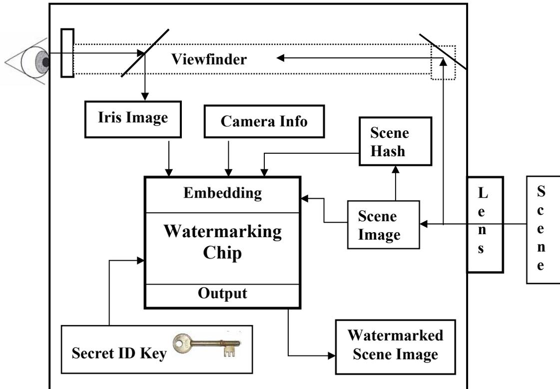
Figure 4. Secure Digital Camera (block diagram).
