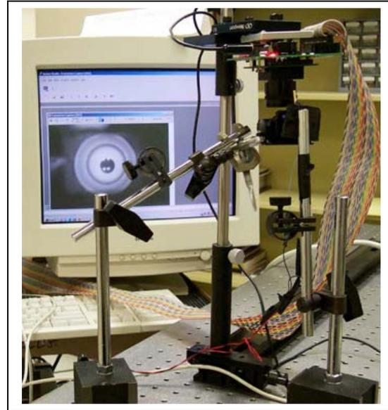
Figure 10. *Iris image capture test setup.*
