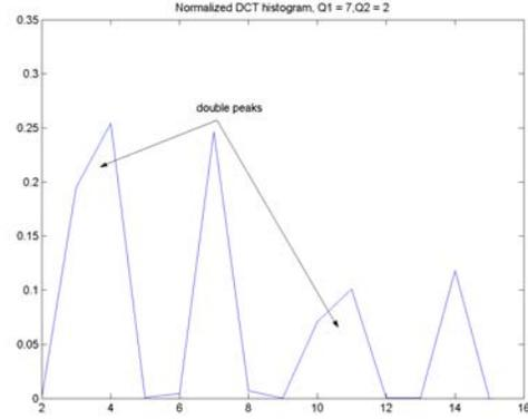
**Figure 1b:** Normalized DCT histogram,  $Q_{ij}^1=7$ ,  $Q_{ij}^2=2$  (ideal case).
