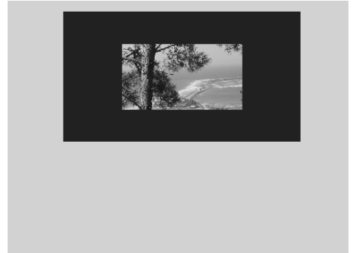
Fig. 4: Top: Detected peak in \text{PCE}(r_i) . Bottom: Visual representation of the detected cropping and scaling parameters r_{\text{peak}}, s_{\text{peak}} . The gray frame shows the original image size, while the black frame shows the image size after cropping before resizing.
