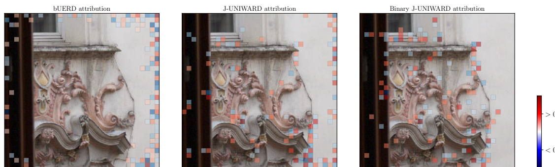
Figure 10. Attribution maps for image ‘43201.jpg’ from the ALASKA II dataset embedded with J-UNIWARD and bUERD from the multi-class, and binary J-UNIWARD EfficientNet B4 (from left to right). Notice the anti-correlated attributions in the right boundary of both images from the multi class attributions, which are not visible in the binary attributions. The figure shows only the 90% largest attributions for each map in absolute value for visual clarity.
