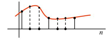
→ Expansion-Filtering is called "<u>Interpolation</u>"
